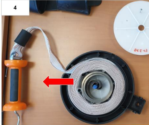
4. Keep the (metal) spring in place and remove the old tape from the reel. Prepare the new tape (max. 15mtr/40mm) by pre-assembling the gate handle and rubber sleeve at the start of the tape.
