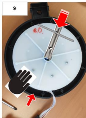
9. Place the transparent reel in the lower part of the black housing. Place the bottom end of the blue shaft in the socket of the black housing, this to secure and maintain the tension on the spring). Keep holding the transparent reel in place! The wrench can be removed now...
