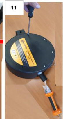
11. Now reassemble the upper part of the outer housing. Make sure the upper part of the (blue) shaft is lined up and locked in the outer housing socket. Now tighten all 8 screws (4 at each side).
