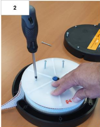
2+3. Take the transparent inner reel out of the outside housing, the tension on the spring will be lost, this is normal.
