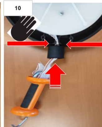
10. Place the tape thru the opening of the outer housing part and guide the last centimeters of the tape gently in the housing until the rubber sleeve in front of the (pre installed) gate handle prevents the transparent reel from further rotating.
