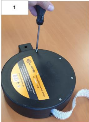
1. Open the outer housing of the reel by removing the 4 screws at each side (8 screws in total)
